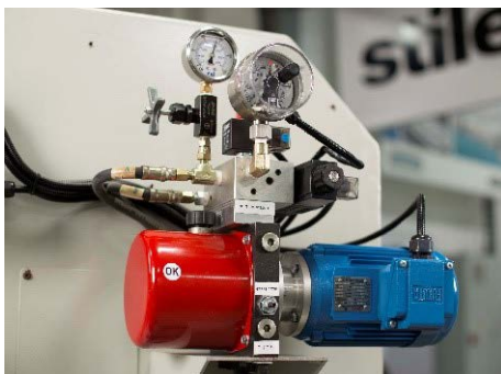
Hydraulic blade tensioning
