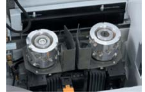
Pre-milling unit with Diamond inserts. 100 mm diameter.
