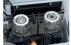
Pre-milling unit with Diamond inserts. 100 mm diameter
