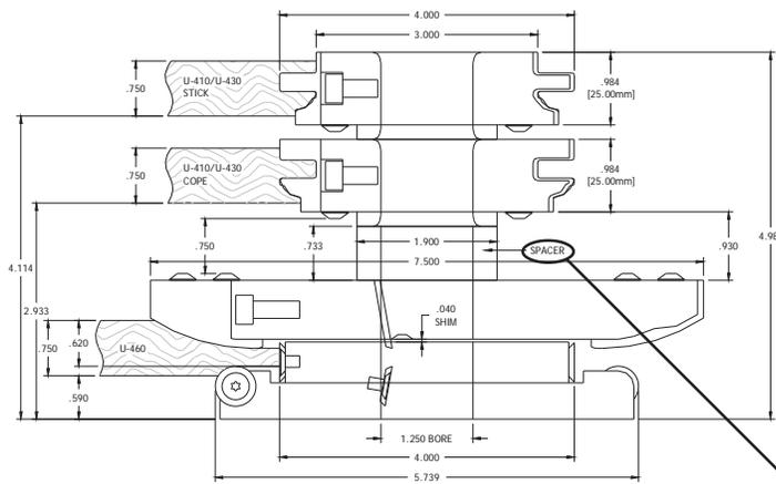
**It is extremely important that this spacer be on the stack between small & large diameter tools.**
