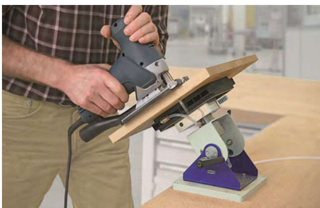
Vacuum clamping system Multi-Clamp can be used to clamp and swivel workpieces directly on the workbench
